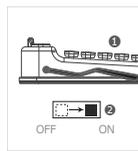
7. Press down and hold the macro bar and turn on the keyboard (keyboard is now in firmware mode)
