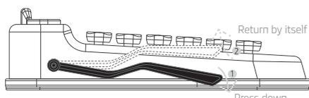
If you press the bar downward slightly, it will return by itself and saved keys are transferred to the tablet PC.
