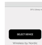
8. Tap on SELECT DEVICE (Search for the target device for the firmware update)
